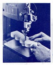
Sanding on irregular pieces is no longer a tedious hand operation if you have this handy attachment for your band saw. Takes but a few minutes to make the change-over from a band saw blade to garnet belt.
