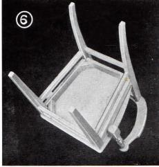
The photo above shows a cutaway view of the chair. The arm support turning is notched and doweled in place in the edge of the seat as shown. The rails are mortised into the legs with the mortising attachment in the drill press. Finish is walnut stain and rubbed varnish.
